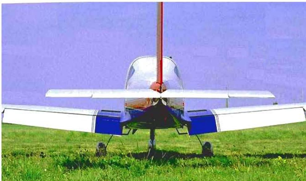
With flaps deployed, a steep approach is possible: a very short flare and roll out will result.
